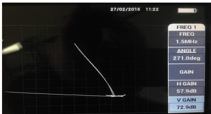
*Typical signal generated over EDM notch 0.50 mm with horizontal lift off*
